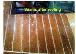
**Seams after reefing:** The seams on the deck have been cleaned and smoothed out.
